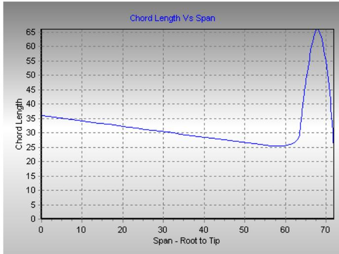
The dialog box shows a plot similar to the one shown at left for a bulb keel. This plot is a very good indication that the design smoothly transitions from along the span. Any unintended odd changes in chord lengths will be shown here.
